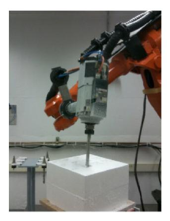
figure 2: industrial robot with milling tool
